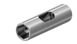
The fastening socket is used for tightening according to the torque of the RollerDrive fastening nut using a torque wrench. The socket features a lateral opening through which the RollerDrive connecting cable can be fed to the outside.
