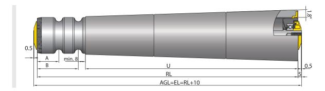
Tapered elements with 1.8° and tube projection on the right
