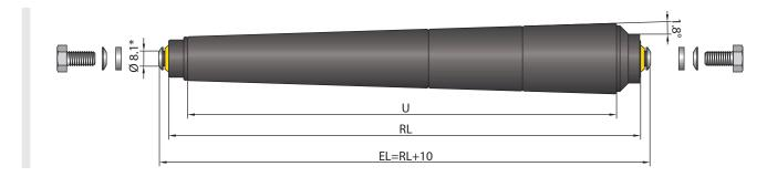
\* The recommended profile holes have a dimension of  $\varnothing$  8.1 mm
